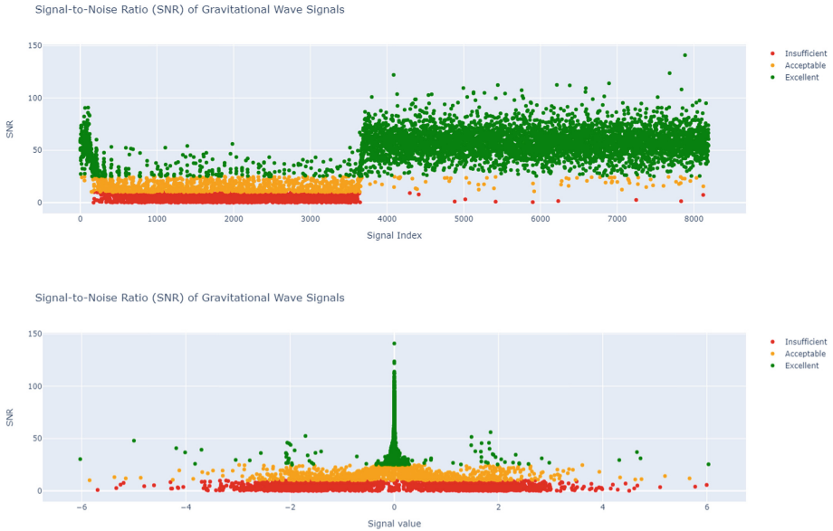
Fig. 2. Top: SNR values by index signal, Bottom: Cleaned signal amplitude
